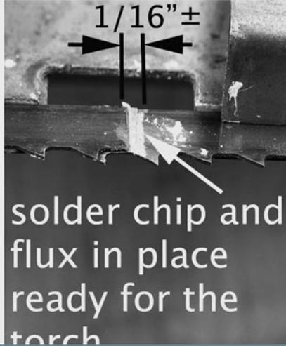
solder chip and flux in place ready for the torch
