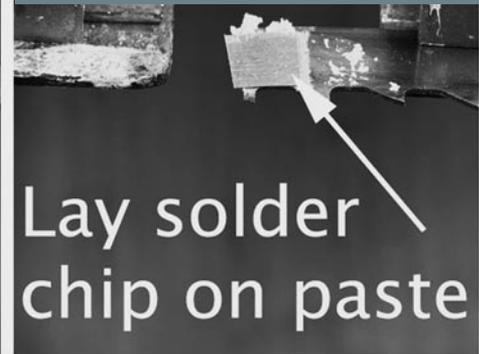
Lay solder chip on paste
