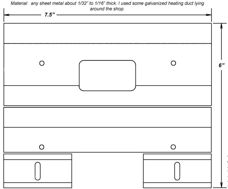
Print out the above pattern on your computer printer and use a glue stick available at any office supply to paste it down to the sheet metal. Cut out by cutting through pattern and paper. After drilling holes (drill holes at end of slots then cut out slot between holes), bending, and making slots (do this in this order), peel off paper pattern. Use alcohol to remove any stubborn paste residue.
