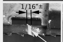
solder chip and flux in place ready for the torch
